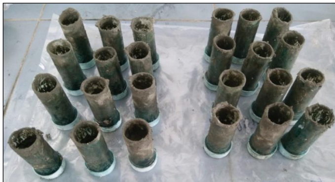
Figure 4. Casting of The Saccharum Officinarum Bagasse Fibres (SOBF) Cement Composite
