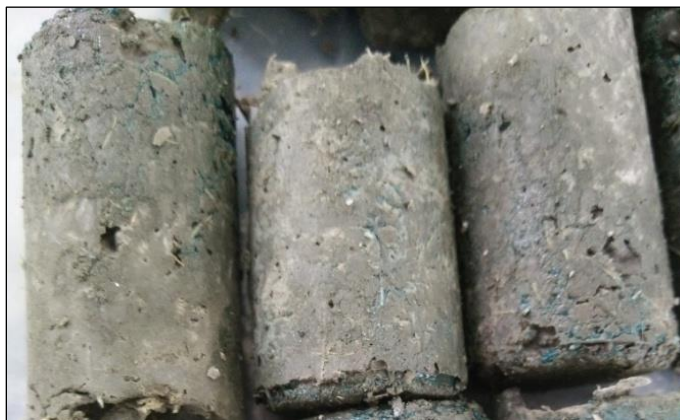
Figure 10. Voids in Hardened Fibre Cement Paste
