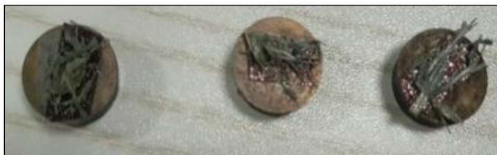
Figure 5. Fibre Treated and Untreated After Coated with Gold
