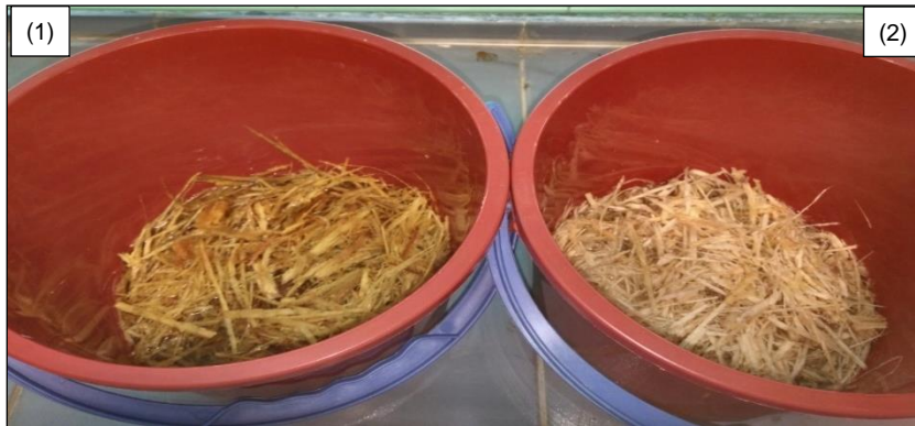
Figure 3. SOBF Soaked Into (1) Alkaline and (2) Acid Solution for 1 Hour
