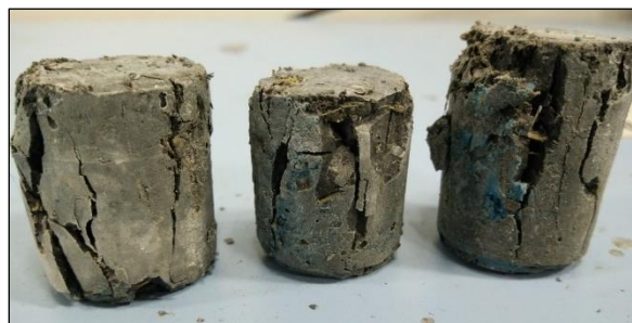
Figure 14. Failure Mode of Rod Specimen Under Compressive Load
