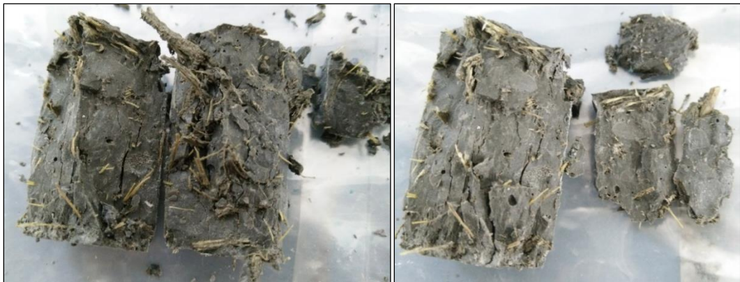
Figure 12. Fibre Inclusion in Hardened Fibre Cement Composite
